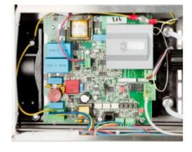
reduce the temperature. A fan blows fresh air over the electronics board and through the heat sinks when the generator is operating. The ONY generators offer adjustable ozone production in two steps, 50% and 100%.
