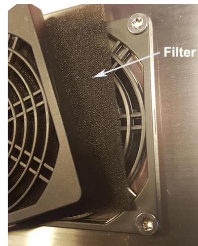
Fig.4 – Filter Cleaning
